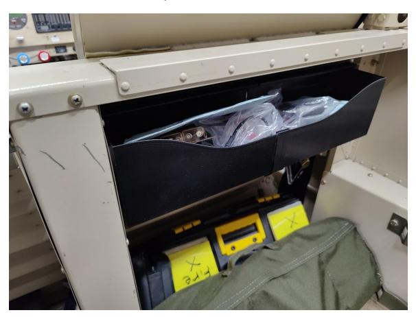
Note: Leave the 3M Dual Lock attached to itself during installation. For installation, only remove the backside adhesive protection.
