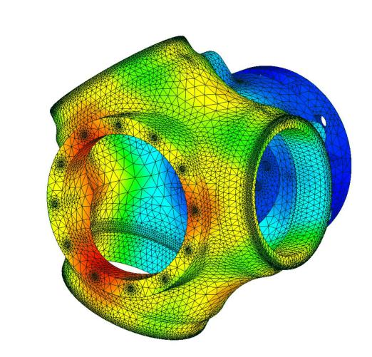
displacement magnitude 0.006944 0.006172 0.005401 0.004629 0.003086 0.003086 0.002315 0.001544 0.0007721 6.947E-07 in Displacement Axial Direction Fwd Face Variation .0068 - .0048 = .002 inch
