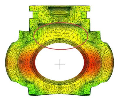
Note: this model assumes an even centrifugal load around the bearing race for simplicity. Because of the hub flex, the load would actually be more concentrated at the aft portion of the race. The aft edge will carry more load because it is stiffer. Upon tear down inspections pay special attention to the aft edge.
