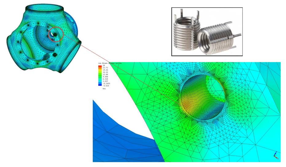
no Cap, von Mises Stress =20 ksi, smooth bore hole no threaded insert, locking tab threaded insert Kt = 3 but area is small and will locally yield and should not present a problem
