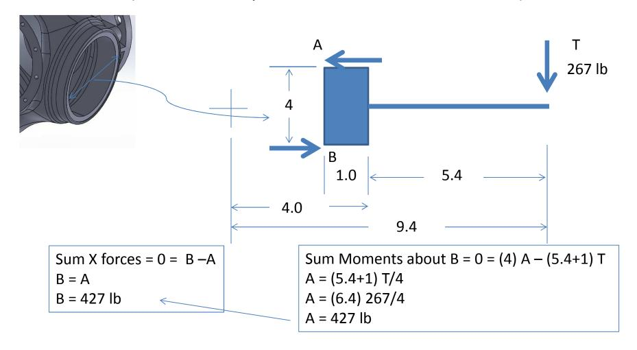
Blade Thrust Component (2835 rpm) (Assumes thrust is located at 50% blade span)
