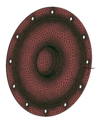
Cap Natural Frequency Model Boundary Condition Fixed at bolt hole ID only
